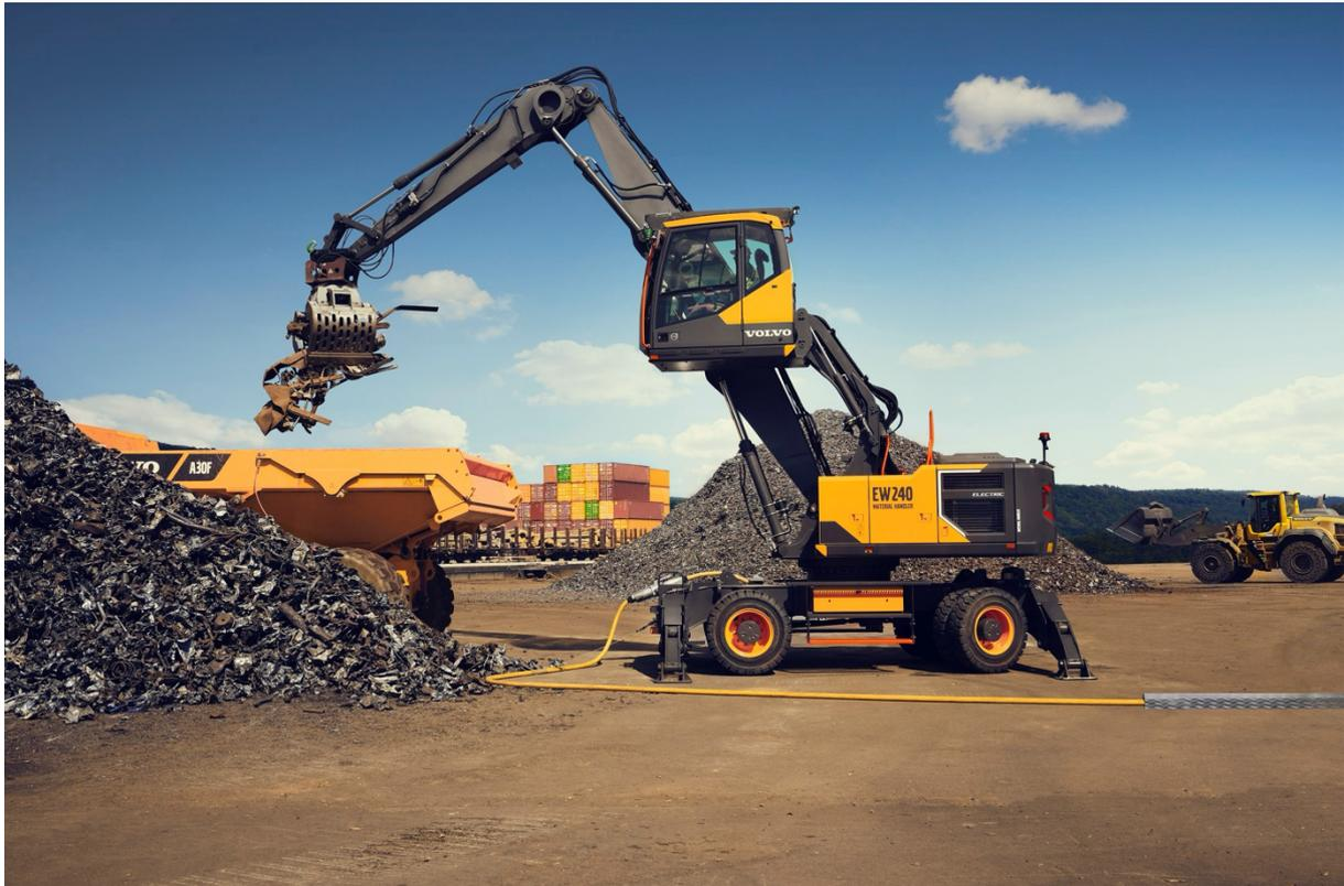
*The grid connected EW240 Electric material handler launched in early 2024, initially for selected customers in Europe.*
