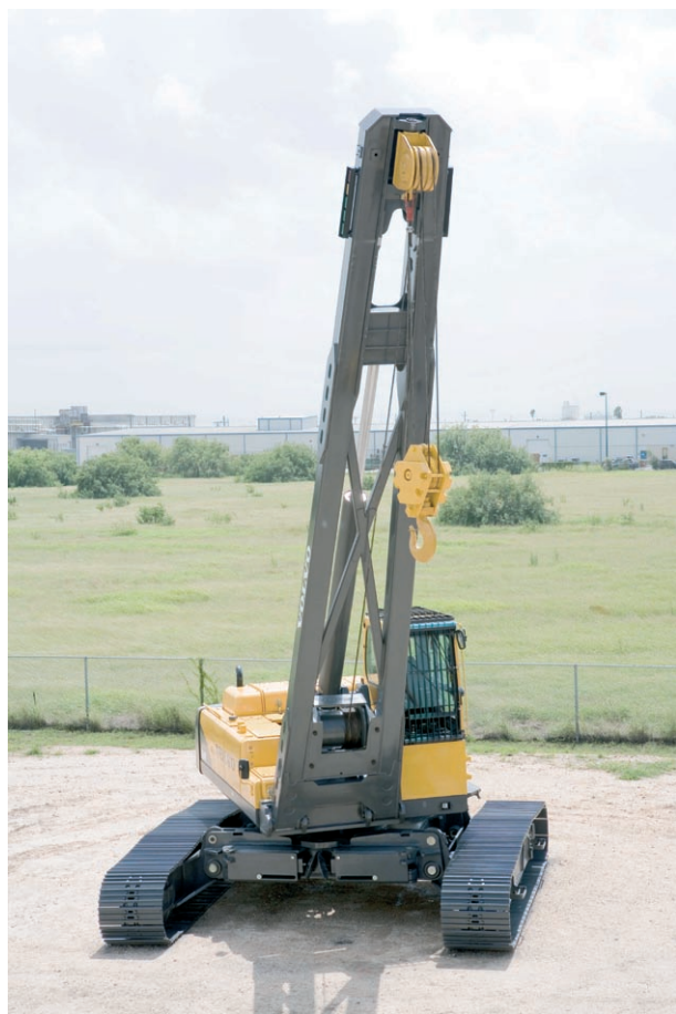
A special purpose lower frame and track frame system on the larger models provides a nearly square working platform, optimising stability: 5.5 m wide for the PL4611, 7.1 m for the PL7015.
