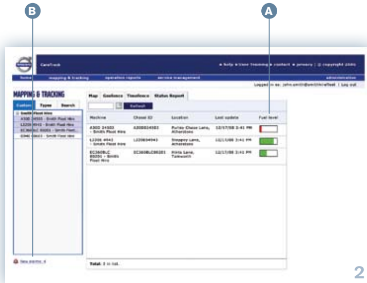
Figure 2: Real-time status and fuel level report
