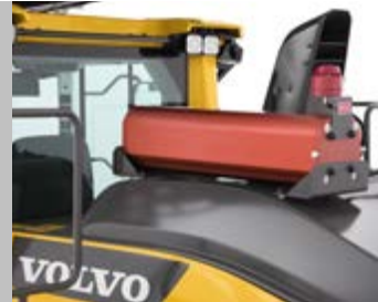
Fire suppressions system
