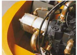
Separate hydraulic pumps provide fast cycle times.
