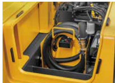
Fuel fill pump
