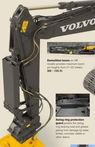
**Boom Cylinder Protection System** visible through the plate from the cabin for visibility to the right track.
