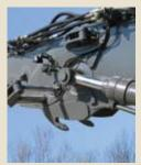
Innovative hydraulic modular joint uses a hydraulic lock mechanism to release digging equipment and change from high reach demolition boom to a standard backhoe configuration in less than 30 minutes. The feature greatly enhances versatility.
