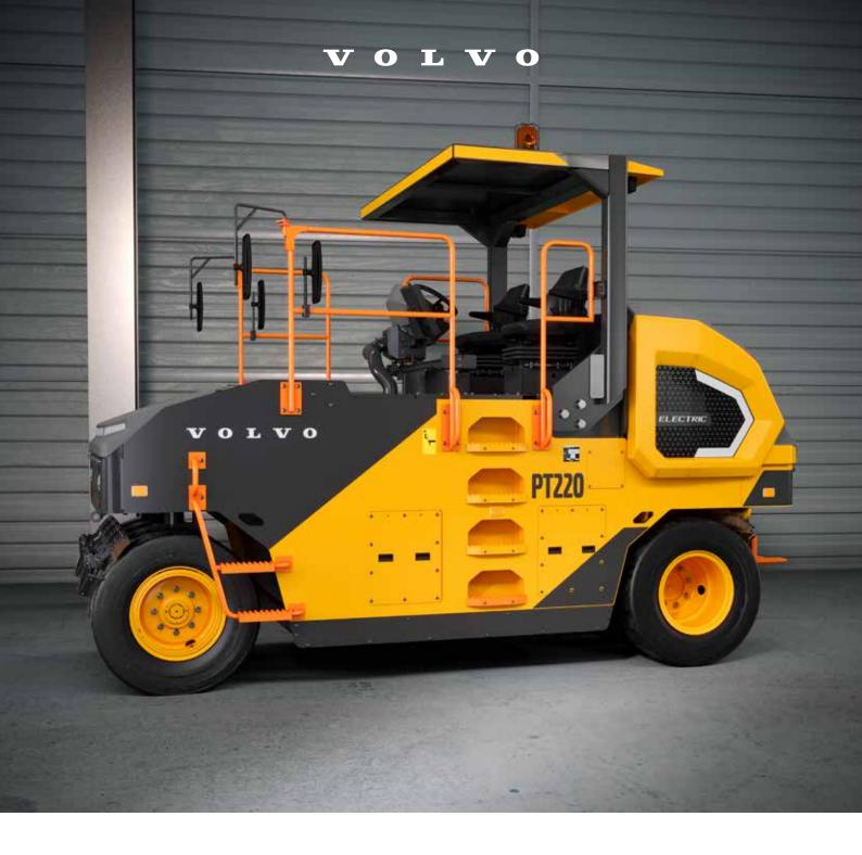
Volvo Pneumatic Tyre Roller 11.0-24.0 t 114 kW
