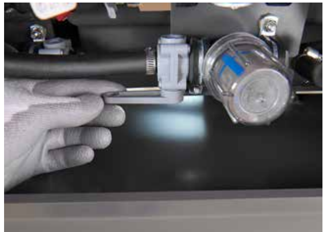
Quick drain freeze prevention
