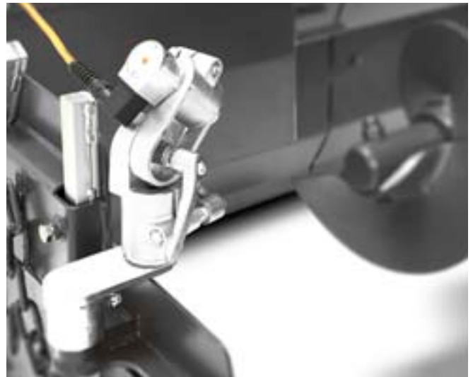
Ultrasonic sensors for proportional auger speed control
