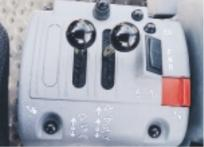
Pilot operated fingertip hydraulic levers provide easy control of the hydraulic functions. The adjustable hydraulic lever console also features a rocker switch for foward/reverse shifting and 1<sup>st</sup> gear kickdown button.
