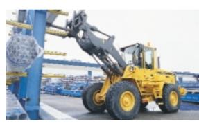
The visibility-optimized attachment bracket and refined TP linkage provide a clear view of both attachment and load.
