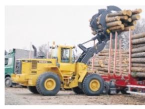
TP linkage comes into its own in logging applications. No other system can provide such high breakout torque throughout the entire lift cycle.
