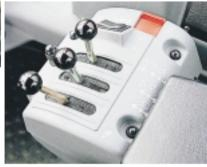
Pilot operated fingertip hydraulic levers provide easy control of the hydraulic functions. The adjustable hydraulic lever console also features a rocker switch for foward/reverse shifting and a 1st gear kickdown button.
