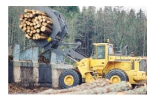
TP linkage comes into its own in timber applications. No other system provides such high breakout torque troughout the lift cycle.
