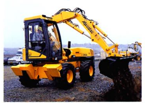
Backfilling at an angle of 90°: the driver faces the work area
