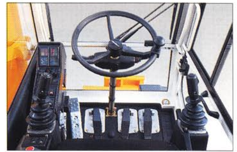
Rops and Fops cab, comfortable, sound-proofed, with excellent visibility.
