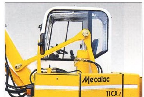
Boom ram with parallelogram frame ensuring variable throw.
