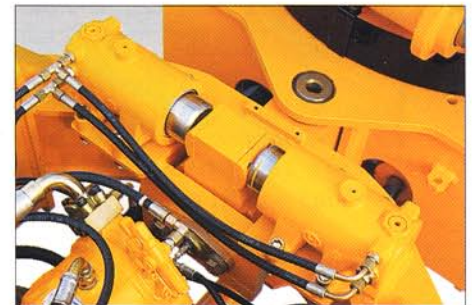
Chassis oscillation lock standard on 11CXi, optional on 11CX model.
