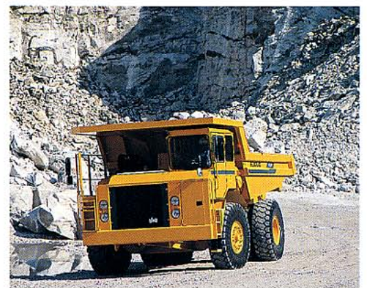
Euclid R32, the Little Giant, carries 1,41 times its own weight. It is a highly productive hauler with low operating costs and therefore low cost per ton transported.
