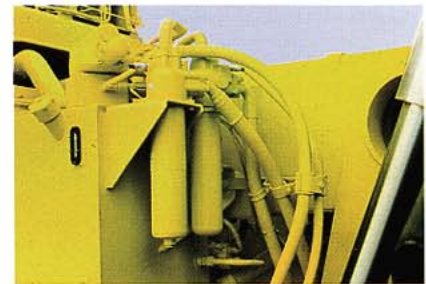
For simple, time-saving serviceability, the lube and fill points on Euclid haulers are positioned for convenient ground level servicing.
