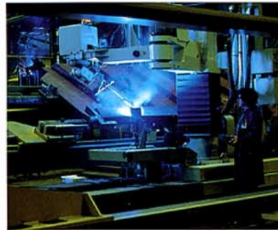
Robotic Welding at Guelph
