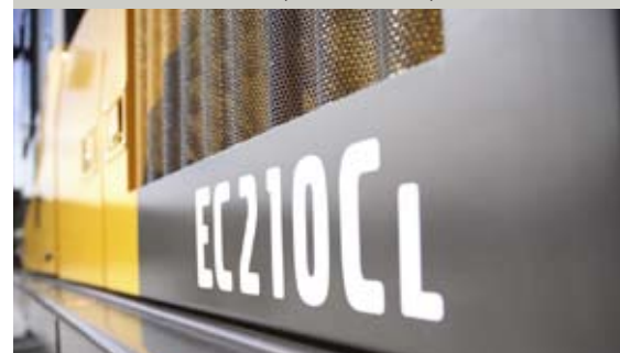
• Micro mesh screens keep particles from coolers.
