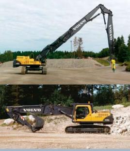
• Easily change from demolition configuration to straight boom or regular backhoe.
