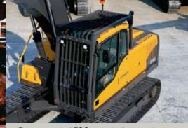
• Frame-mounted FOG protects the operator.
