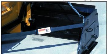
Augers: Two independently operated 10" augers w/ forward and reverse operation to aid in moving material back into screed area / mounted on tractor / automatic or manual modes.
