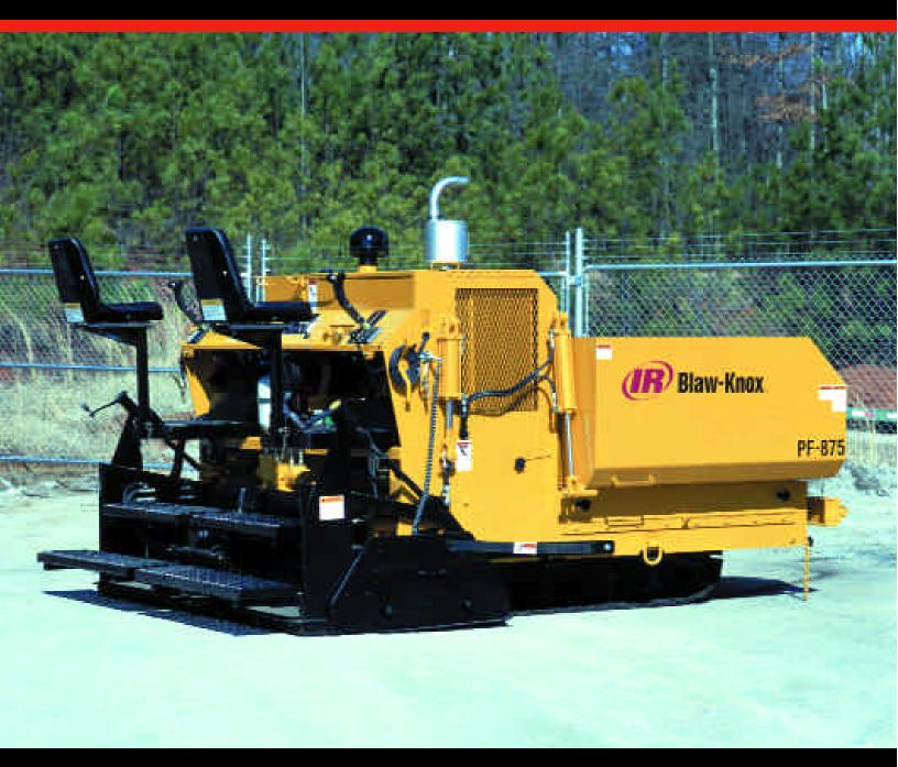
The PF-875 is a track mounted paver/finisher with standard paving widths of 8 to 13 ft and optional bolt on extensions for paving up to 15 ft. The material delivery system is a 8 ton capacity automatic dual conveyor system. The PF-875 is equipped with many of the same features found on Blaw-Knox highway class pavers and is designed for high efficiency on large commercial jobs. Typical applications include driveways, secondary roads, large commercial parking lots and municipal work.
