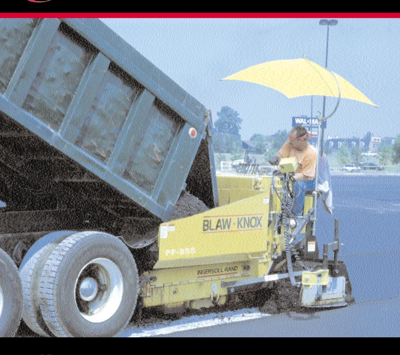
The **PF-855** is a track mounted paver/finisher with standard paving widths of 8 to 12 ft. The material delivery system is a 7 ton capacity automatic dual conveyor system. The PF-855 is designed for high efficiency on large commercial jobs. Typical applications include secondary roads, commercial parking lots and drives.
