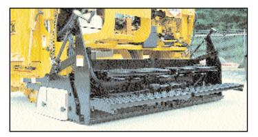
**Augers:** Two independently operated 10" augers w/ forward and reverse / mounted on tractor / automatic or manual operation.
