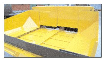
**Paving Depth:** 0-6" / manually adjustable with two bearing-free depth adjustment jacks. Depth indicators are standard.
