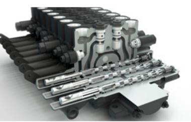
**Custom designed spools and load-sensing hydraulics.** The load-sensing hydraulic system balances flow to all grading functions. It is optimized through the use of custom designed spools in the main control valve – permitting precise blade control, fast response and smooth operation at all speeds.
