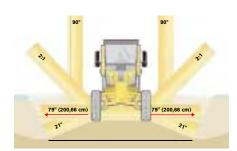
The MBCS gives you the flexibility to position the blade at any angle you need for shouldering, slope work and ditch cleaning – up to 90° upward and 21° downward.
