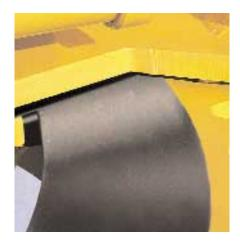
Duramide™ bearing material eliminates metal-to-metal contact and reduces the need for circle turn lubrication and adjustment. As well as being simple and costeffective to replace, it has a minimum service life of more than 5,000 hours.
