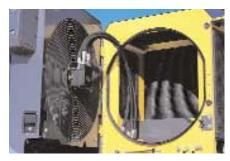
Since the grader's need for cooling depends on ambient conditions as well as the engine's power output, the variable-speed hydraulically driven fan on Volvo graders is designed to respond to actual demand. Combined with non-stacked coolers, the system continuously delivers just the right amount of cooling effort, consuming less fuel, producing less noise and maximizing available power for other grader functions.
