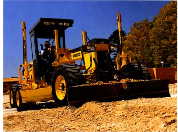
All Volvo Motor Graders are easily fitted with Automatic Blade Control systems for fast and precise fine grading
