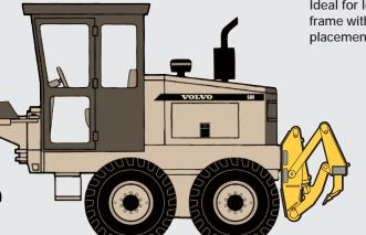
Ideal for loosening hard packed aggregate surfaces. Mounted to the rear frame with standard attachment brackets. Shanks are easily removed and placement locations allow for single tooth ripping.
