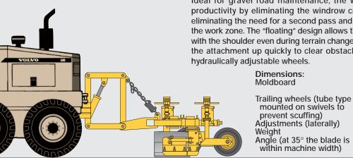
Ideal for gravel road maintenance, the Windrow Eliminator increases productivity by eliminating the windrow created when grading, thereby, eliminating the need for a second pass and reducing the time spent to flag the work zone. The "floating" design allows the attachment to stay in contact with the shoulder even during terrain changes. The parallel lift system brings the attachment up quickly to clear obstacles. Available with manually or
