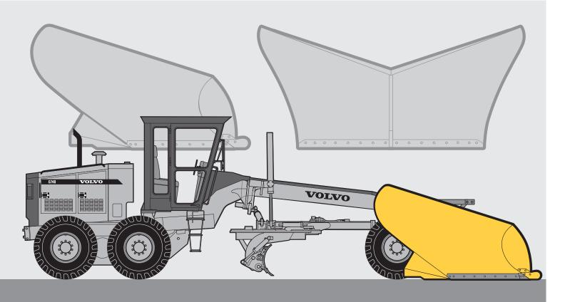
The Volvo "V" Snow Plow is designed for severe snow clearing applications such as opening uncleared roads. The "V" plow slices the material and displaces the snow in both directions for maximum single pass snow clearance at high speed.
