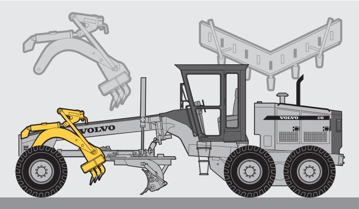
A scarifier attachment is designed to break up compacted material, asphalt, rocky subgrade to facilitate grading.
