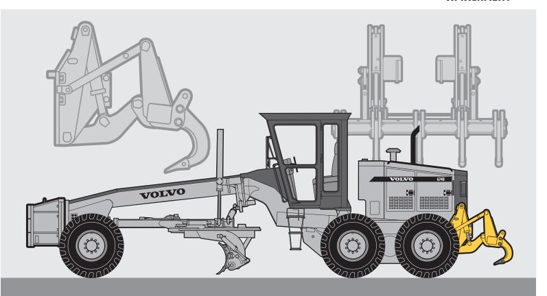
The Volvo Ripper/Scarifier is a rear mounted tool used for tearing up asphalt, hard-pack or other obstacles to aid the grading operation.
