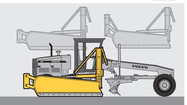
The Volvo Hydraulic Snow Wing is designed for high or low speed snow clearing application in combination with the grader moldboard or snow plow as the primary plowing tool. As material is displaced from the snow plow, the snow wing is designed to displace the material far back from the road surface to eliminate snow buildup and facilitate continued snow displacement.
