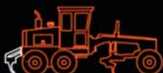
Rear Ripper: rear mounted, 5 tooth; ideal for tearing up sealed surfaces and site clearing.
