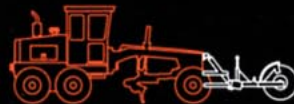
Broom for rapid clean-up of intersections, aggregate removal from sealed surfaces, and final clean-up after asphaltting.
