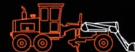
Loader; fewer machines needed for site clean-up and clearing. Load height sufficient for tandem dump truck.
