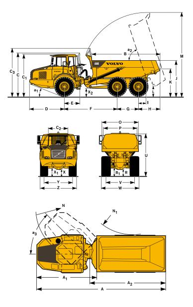
A25E: Unloaded machine with 23,5 R25 A30E: Unloaded machine with 750/65R25 \*) A30E with optional 23,5 R25 tires
