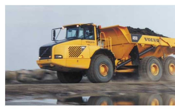
The front axle's sturdy rubber suspension with shock absorbers means that it can maintain high average speeds while preserving operator comfort and minimizing mechanical wear. The bogie design means that each pair of wheels can move independently to maintain ground contact. This lets the body move practically horizontally over irregularities in the ground while the frame undergoes less stress.
