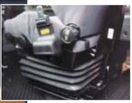
An air suspension operator's seat improves comfort.
