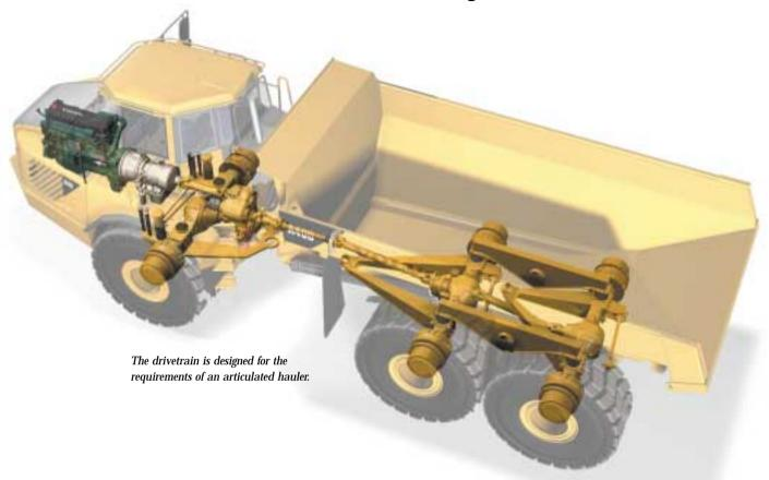
The reason that the articulated hauler is so successful in performing its tasks is that the drivetrain is finetuned and optimized for its job. Volvo's articulated haulers have always been characterized by a drivetrain that is designed for the specific requirements of an articulated hauler.
