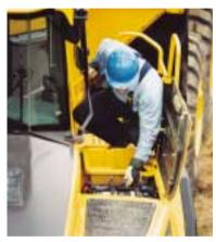
The batteries are easily accessed next to the storage compartment.
