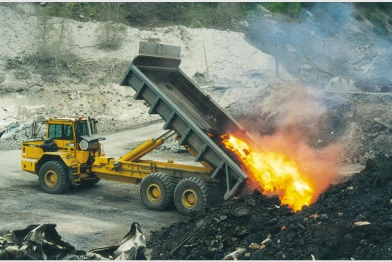
An A30C 6x6 Hook Lift is used by Horn & Co. for Krupp (Edelstahlprofile) GmbH in Siegen, Germany. It is used primarily to haul slag, but can also be used for other types of haulage at the steel mill thanks to its interchangeable loading system.
