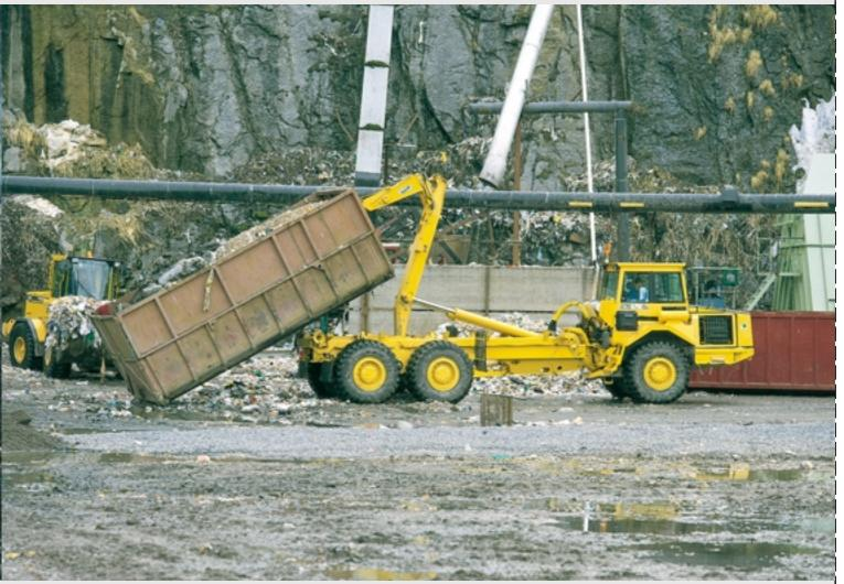
An A25C Hook Lift at a recycling facility in Vaasa, Finland. With the interchangeable loading system the same vehicle can be used for many different jobs.
