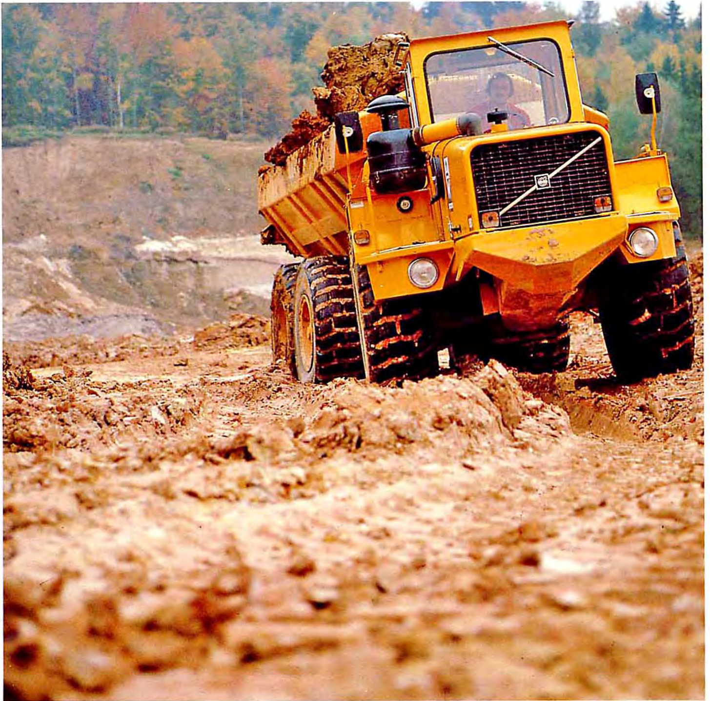
The dumper shown on the illustration is equipped with an extra oil bath air cleaner.
