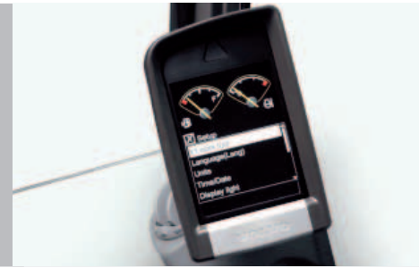
Hammer & shear: variable flow and pressure pre-setting
