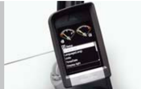
Hammer & shear: variable flow and pressure pre-setting
