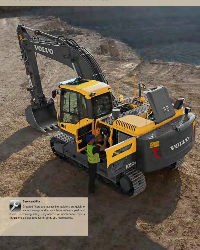
With built in serviceability the new Volvo D-Series crawler excavators guarantee you more uptime. Easy access to grouped service points allows for fast and effortless maintenance and service checks. Achieve more with Volvo.
