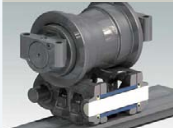
• Lifetime greased and sealed track link.
