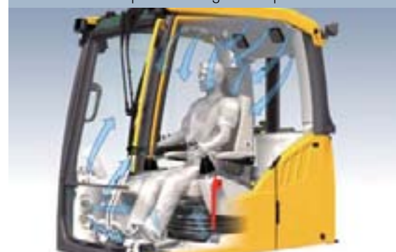
• Industry's highest heating/cooling capacity with 14 vents.
