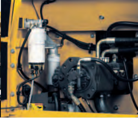
• Easy access for hydraulic pump filters.
