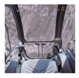
Surrounded by an easy to use console, the seat has eight simple adjustments for maximum comfort and working visibility, whether in deep trenching or truck loading.
