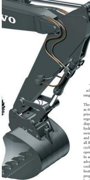
A state-of-the-art hvdraulic system performs as a direct extension of the operator's thoughts and movements. That's why the Bseries hydraulic system is designed with operator controllability and precision as its focus. With four different power modes, B-series hydraulics respond automatically to the operator's joystick movements and pilot pressure. This allows Volvo machines to achieve maximum efficiency on a full range of jobsites.
