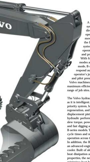
A fine-tuned hydraulic system performs as a direct extension of the operator's thoughts and movements. That's why the B-series hydraulic system is designed with operator controllability and precision as its focus. With four different power modes and a power max mode, B-series hydraulics respond automatically to the operator's joystick movements and pilot pressure. This allows Volvo machines to achieve maximum efficiency on a full
