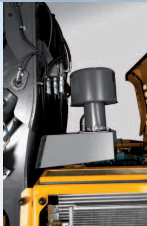
• Pre engine cyclone filter
