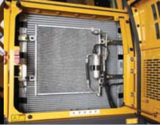
• Reversible cooling fan with sealing
