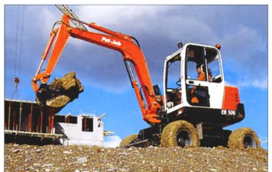
The equipment offset pivot, based on the double fork technique, minimises equipment play and means that the hoses at the base of the boom can be quickly changed.
