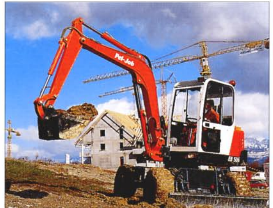
The EB 506 P is equipped with a mechanical slewing brake to eliminate any risk of drifting when working on a gradient.
