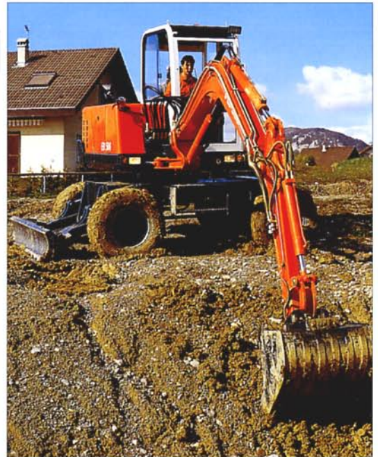
Two dipper arms available for deep digging tasks: 3133 mm with 1500 mm arm and 3533 mm with 1900 mm arm.
