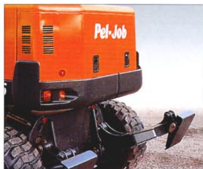
New streamlined hood and tank design. Engine cover guard built into counterweight. Large capacity diesel fuel tank providing a large autonomy without refuelling. Volume of hydraulic oil tank optimised to reduce maintenance costs.
