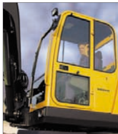
Thanks to its compact dimensions and the boom's hydraulic offset, the EW70 is at ease in all site configurations, even alongside a wall.
