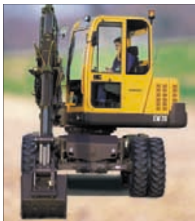
Thanks to its compact dimensions and the boom's hydraulic offset, the EW70 is at ease in all site configurations, even alongside a wall.
