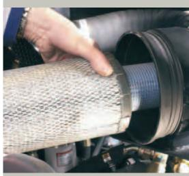
Two-stage air filtration system eliminates need for pre-air cleaner and helps increase engine life.
