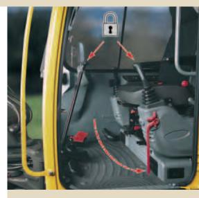
All controls lock out when safety lever is lowered.
