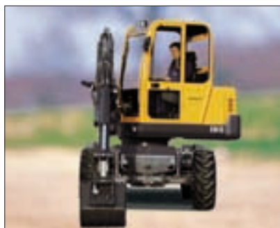
Thanks to its compact dimensions and the boom's hydraulic offset, the EW50 is at ease in all site configurations, even alongside a wall.
