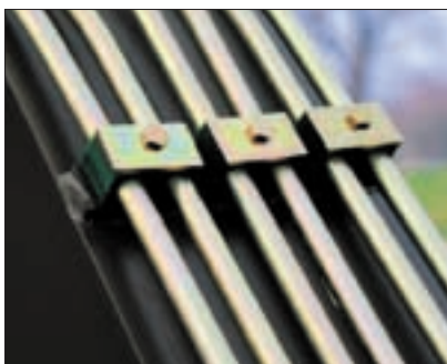
Very effective corrosion protection : all the nuts and bolts, the pins and the hydraulic pipes are zinc-plated.
