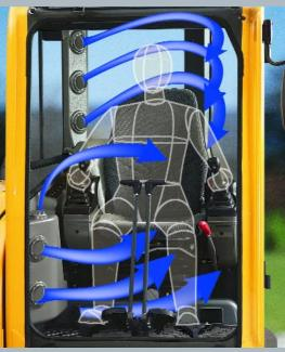
Heating and air-conditioning keep operator comfortable.
