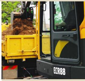
Open door is protected in the width of the chassis.
