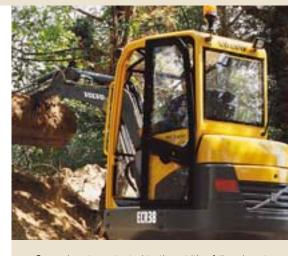
Open door is protected in the width of the chassis.
