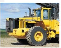
Openable engine access doors with gas struts and swing-out radiator grille and radiator simplify service and cleaning.
