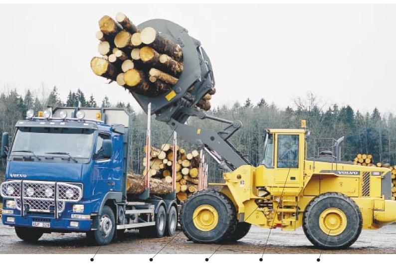
Volvo's patented TP liftarm system positions the load's centre of gravity near the front axle. Stability increases and the tipping load is fully utilized. The front axle is equipped with 100% differential lock.
